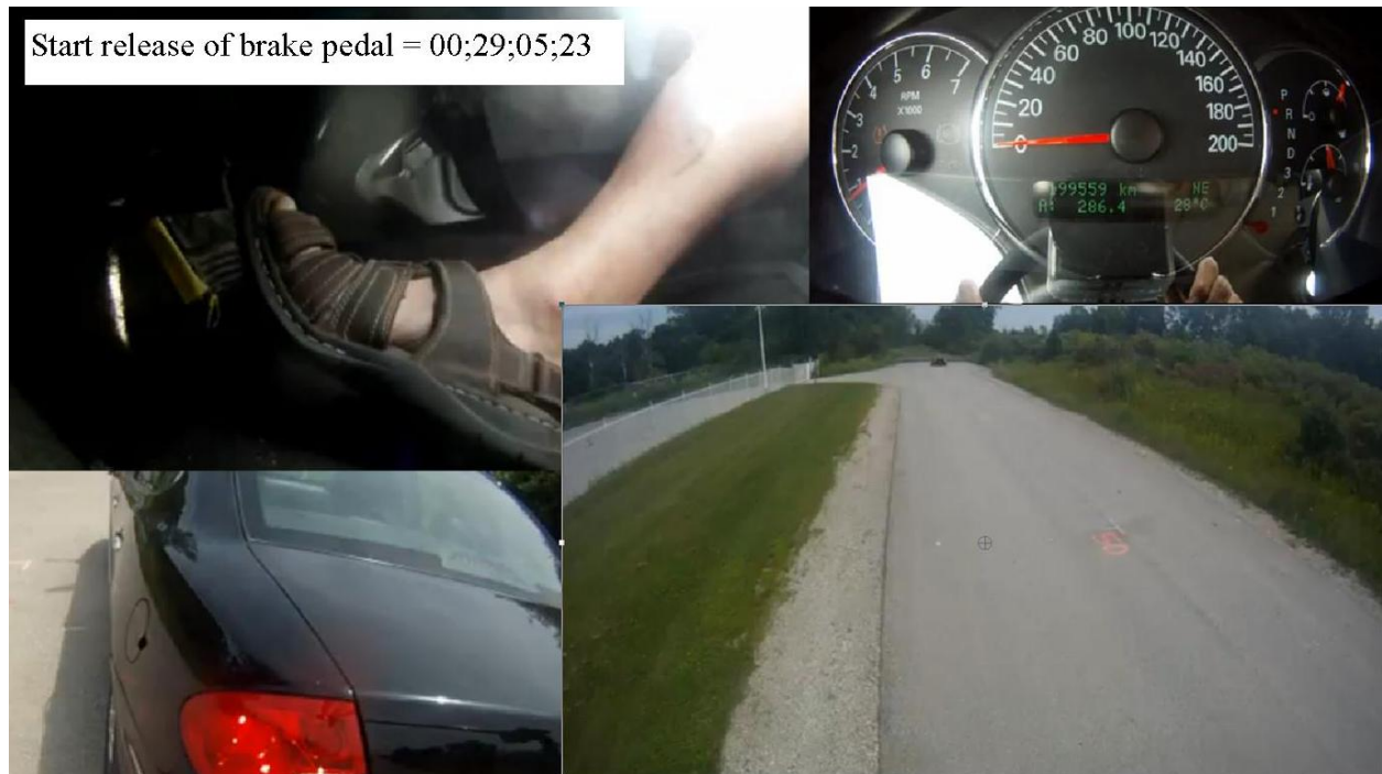
Figure 9: Views from four video cameras at the start of Test #1. In the upper left is a view of the driver's foot at the time that it began to release the brake pedal. The status of the speedometer and tachometer can be seen in the upper right. The view from a camera positioned near the 50-metre marker is shown in the bottom right. The view of the exterior braking lights of the test vehicle is shown in the bottom left.
